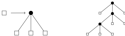
FIGURE 1. A construction rule of a D -ary tree with D = 3 and an example of its realization at time n = 3 .
